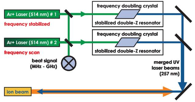
Figure 2: Laser system used for laser-cooling. The frequency of one laser beam is scanned relatively to the fixed frequency of another laser system. The scanning is controlled by measuring the beat signal of the two laser beams. Both laser beams are frequency-doubled separately using beta-barium borate crystals placed in a double-Z resonator geometry. After frequency-doubling, both beams are merged to one and brought in overlap with the ion beam.
