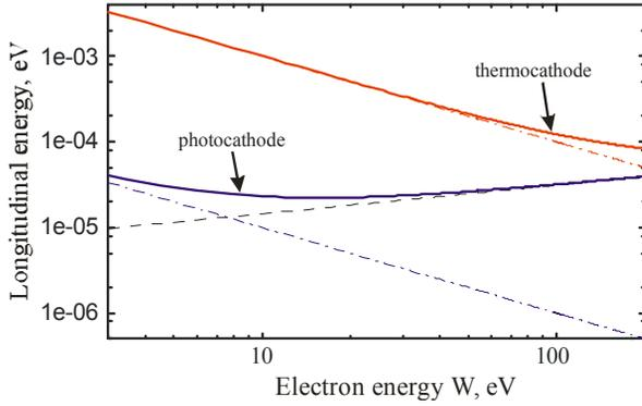
Figure 1: Longitudinal temperature vs electron energy for thermocathode and photocathode electron beams. The kinematic (dashed-dotted lines) and density (dashed line) terms of the Eq. 2 are also shown.
