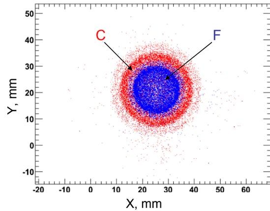
Figure 4: Image of C and F neutral fragments of the cooled ion beam after 12 s.
