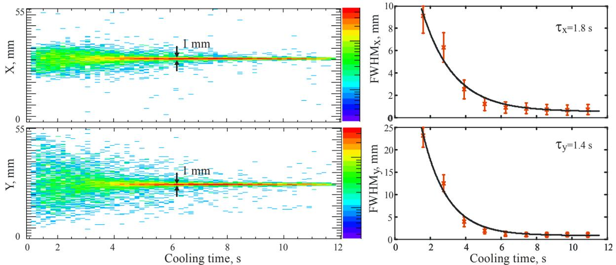
Figure 5: Transverse electron cooling of 97 keV/u  $CF^+$ . Centre-of-mass positions of the C and F neutral fragments vs time, recorded 12 m downstream of the electron target by the imaging detector and indicating rms divergence angles of about  $3 \cdot 10^{-5}$ .
