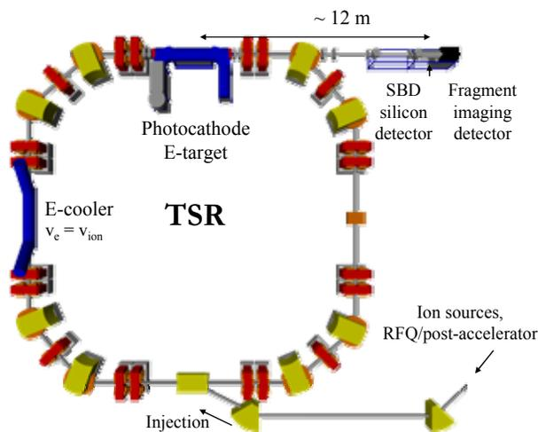
Figure 3: Layout of the Heidelberg Test Storage Ring.
