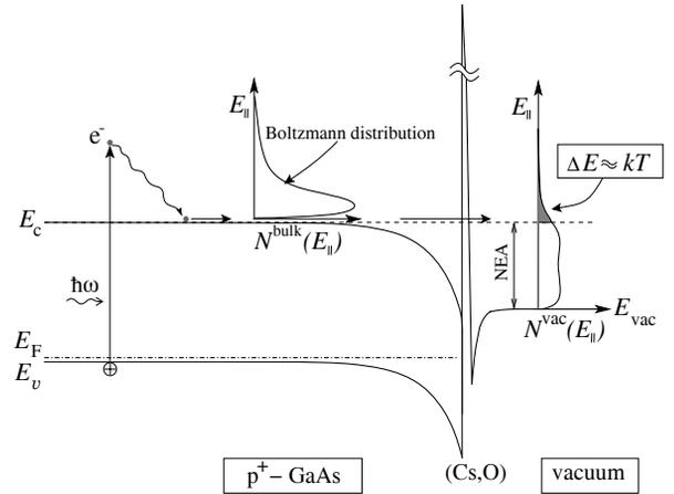
Figure 2: Band diagram of NEA GaAs schematically illustrating the photoemission process.
