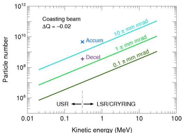
Figure 2: Space charge limit in LSR/CRYRING and USR for a coasting beam with  $\Delta Q = -0.02$ . The crosses represent the maximum number of protons that could be accumulated in CRYRING and the maximum number that has been decelerated.
