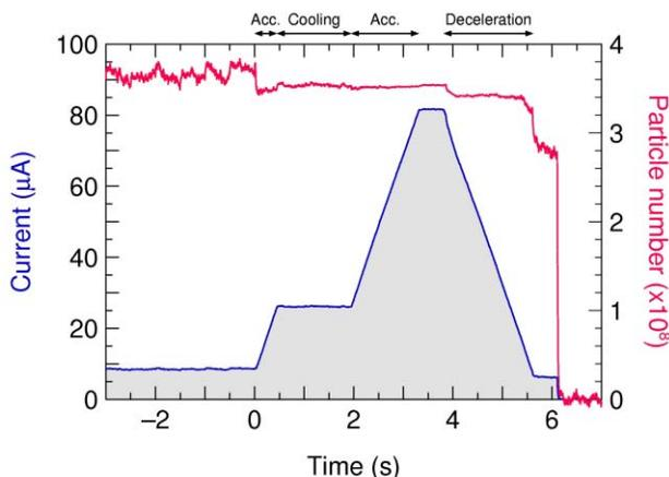
Figure 6: Proton beam current and particle number as in fig. 5 but at higher beam intensity.
