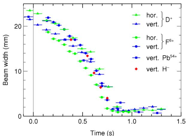
Figure 4: Transverse cooling times of positive ions with different charge states [5] and of  $H^-$  ions. The new  $H^-$  data are normalized to the same electron density of  $1.7 \times 10^{13} \text{ cm}^{-3}$  as used for the positive ions, and these were in addition scaled with  $q^{1.7}/A$ . The new  $H^-$  data points were also shifted horizontally so that the beam reaches a cold equilibrium at approximately 0.7 s, as was the case for the positive ions.
