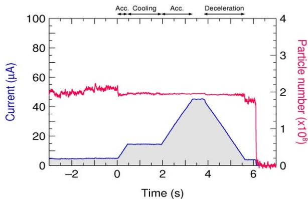
Figure 5: Proton beam current and particle number as functions of time during acceleration and deceleration.
