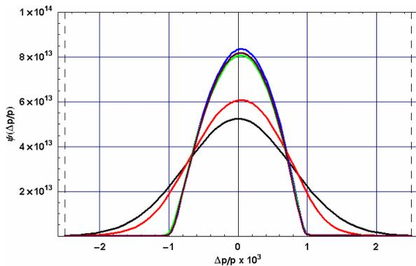
Figure 4: TOF momentum cooling at  $T = 3 \text{ GeV}$  for the HL-mode. The mean energy loss due to the target-beam interaction is compensated. The initial distribution (black) is cooled down to a stable equilibrium without tails in about 300 s (brown curve).
