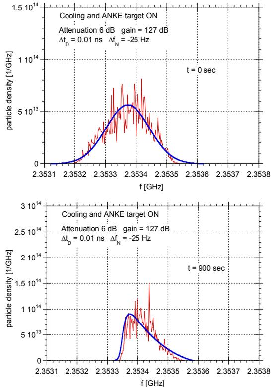
Figure 8: Measured beam distributions (red) during cooling in comparison with model predictions (blue). Initially a Gaussian distribution has been assumed with values for the center frequency and variance determined from the measured initial distribution.
