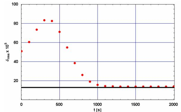
Figure 3: Rms-relative momentum spread (red dots) during cooling with an internal target at  $T = 3\text{ GeV}$  for the HL-mode. Horizontal line: eq. (2)
