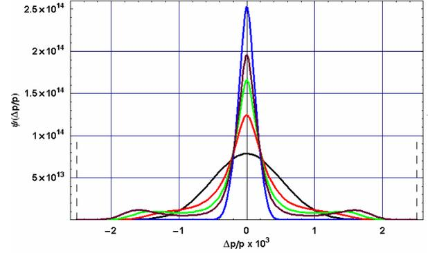
Figure 2: Beam distributions at  $t = 0\text{ s}$  (black),  $50\text{ s}$ ,  $100\text{ s}$ ,  $150\text{ s}$ ,  $2000\text{ s}$  (blue) for the HL-mode at  $T = 3\text{ GeV}$ . The mean energy loss is assumed to be compensated. The acceptance limit (dashed lines) is  $\pm 2.5 \cdot 10^{-3}$ .
