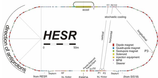
Figure 1: Layout of the HESR ring including the signal paths for transverse and longitudinal cooling.
