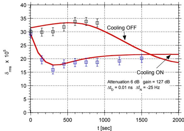
Figure 6: The measured relative momentum spread at harmonic 1500 (blue symbols: cooling ON, black symbols: cooling OFF) in comparison with the model predictions (red curves). The linear increase of the squared momentum spread determines the mean square relative momentum deviation per turn when cooling is switched off.
