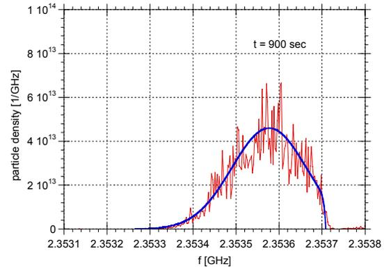
Figure 7: Measured frequency distributions (red) at harmonic number 1500 for  $t = 900$  s in comparison with the model prediction (blue curve). The sharp cut-off at about 2.3537 GHz corresponds to the acceptance limit.
