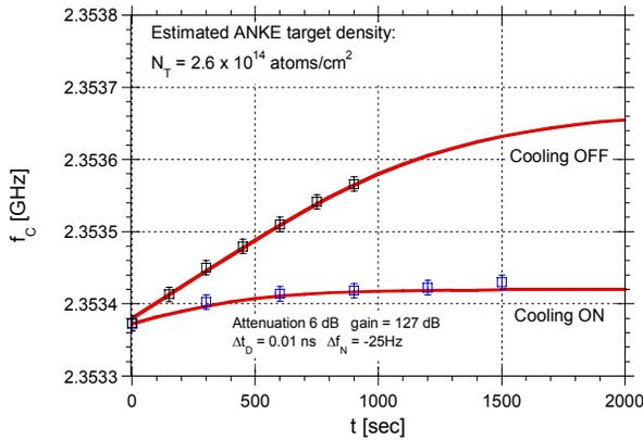
Figure 5: The measured center frequency at harmonic 1500 (blue symbols: cooling ON, black symbols: cooling OFF) in comparison with the model predictions (red curves).
