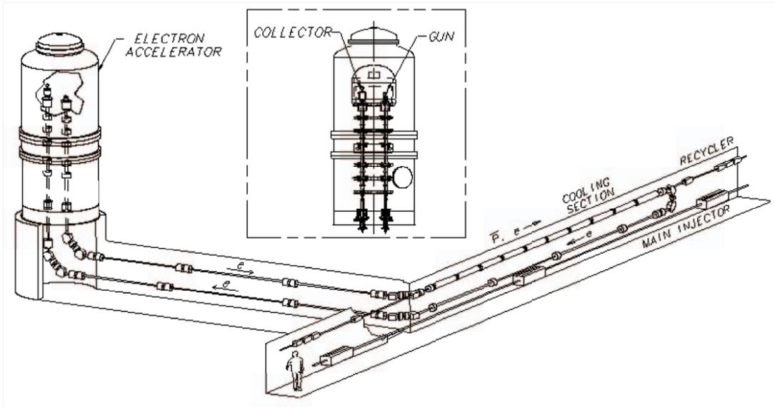
Figure 2: Electron Cooling insert in the Fermilab Recycler.
