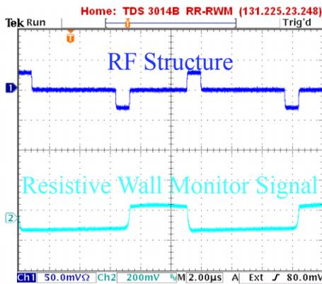
Figure 4: An oscilloscope view of the RF waveform (the integral creates a potential well) and the resistive wall monitor signal. The Recycler revolution period is  $11.13 \mu\text{sec}$ , so the  $20 \mu\text{sec}$  displayed shows more than 1 full turn.
