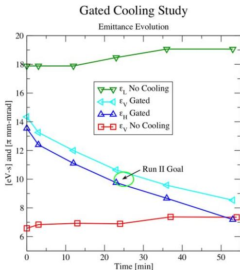
Figure 1: Gated cooling demonstration for the stochastic cooling systems.  $20 \times 10^{10}$  antiprotons were in a barrier potential well and the transverse stochastic cooling systems were gated to cool only the particles in that well. An additional  $20 \times 10^{10}$  antiprotons were in a separate potential well and were not cooled. The goal was to cool to  $10\pi$  mmmrad within 30 minutes. The goal was attained, with no heating to the beam that was not in the cooled potential well.
