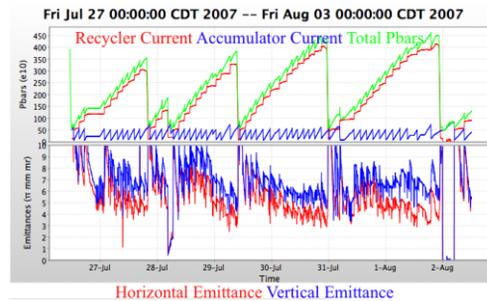
Figure 3: An operational week for the Recycler. In the top plot, blue is the Accumulator intensity, red is the Recycler intensity, and green is the sum (in units of  $10^{10}$ ). In the bottom plot, red is the horizontal transverse emittance and blue is the vertical transverse emittance (both 95% normalized  $\pi$  mm mrad).
