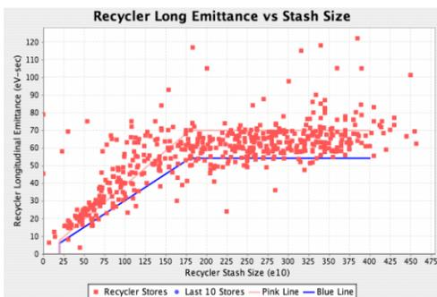
Figure 6: The calculated 95% longitudinal emittance (in units of eV-sec, assuming a Gaussian beam distribution) for the Recycler as a function of the beam intensity (units of  $10^{10}$ ). The pink and blue lines represent performance goals for cooling performance.
