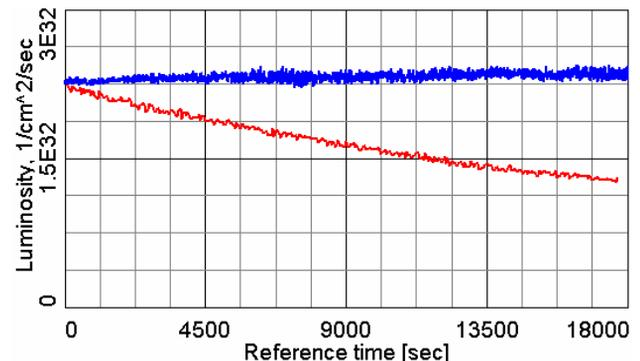
Figure 5: p-p luminosity at 100 GeV for ion bunch intensity  $2 \times 10^{11}$  and 111 bunches, using two 5nC electron bunches. With (upper blue curve) and without (low red curve) electron cooling, respectively.
