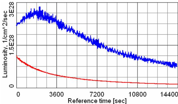
Figure 2: Simulation of Au-Au luminosity for ion bunch intensity  $2 \times 10^9$  and 111 bunches using two 5nC electron bunches per single ion bunch with (blue top curve) and without (red bottom curve) electron cooling, taking  $\beta^*=0.5$  m and 1 m, respectively.
