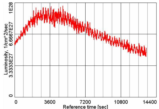
Figure 1: Electron cooling simulation of Au-Au luminosity: ion bunch intensity  $1 \times 10^9$ , 111 bunches; using single electron bunch per ion bunch. Average luminosity in 4 hour store is  $7 \times 10^{27} \text{ cm}^{-2}\text{s}^{-1}$ .
