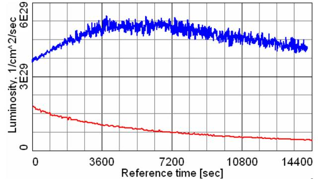
Figure 4: Cu-Cu luminosity for ion bunch intensity  $8 \times 10^9$  and 111 bunches. Average luminosity in 4 hour store  $4.6 \times 10^{29}$  and  $0.8 \times 10^{29} \text{ cm}^{-2} \text{ s}^{-1}$  with (upper blue curve) and without (low red curve) electron cooling, respectively.
