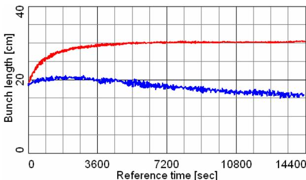
Figure 3: Simulated bunch length for ion bunch intensity  $2 \times 10^9$  using two 5nC electron bunches with (blue bottom curve) and without (red upper curve) electron cooling.
