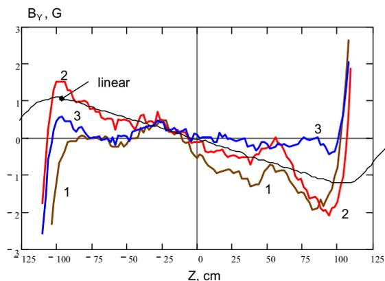
Figure 2: Vertical field before inclination of margin coils - 1, and after - 2, compensation with linear corrector; linear - a field of the linear corrector with an opposite current.
