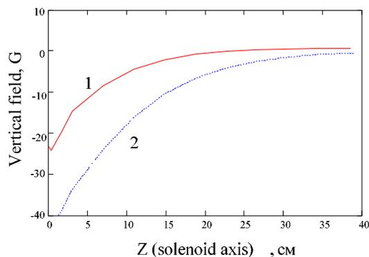
Figure 3: Vertical field distribution at solenoid and toroid junction: 1 - with magnetic diaphragm, 2 - without it.
