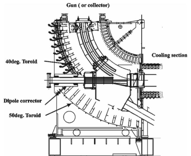
Figure 5: Dipole corrector inserted into 50 deg. bending section.
