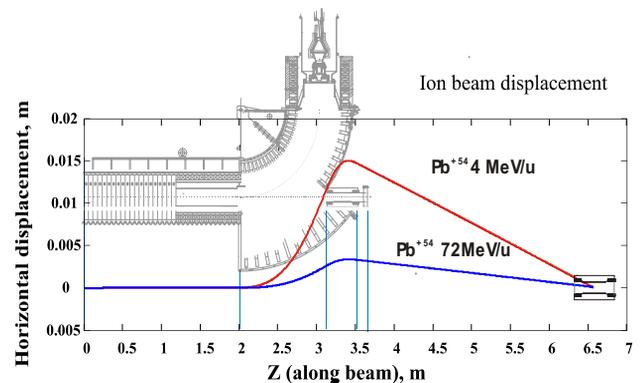
Figure 6: Scheme of correction of ion beam orbit.
