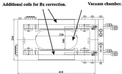
Figure 7: Design of the dipole corrector.
