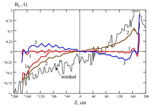
Figure 1: Vertical fields at cooling section of EX-300 measured at longitudinal field: curve 1: 0.75 kG, curve 2: 0.5 kG, curve 3: 1 kG. Curve 1a: 1-st switching on after return to a field of 0.75 kG. “Residual” – result of Hall probe measurements of the residual field.
