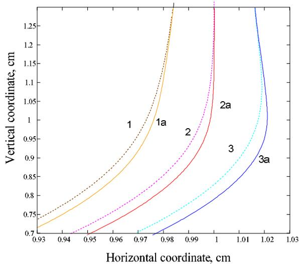
Figure: 4 Results of simulations of electron beam trajectory. 1,2,3 - without diaphragm 1a, 2a, 3a with diaphragm.
