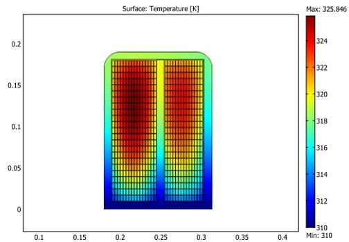
Figure 8: Simulation of temperature distribution in a cross-section of the coil. The temperature of the bottom surface is fixed at 310 K ( $=37^\circ\text{C}$ ). The other surfaces are isolated.
