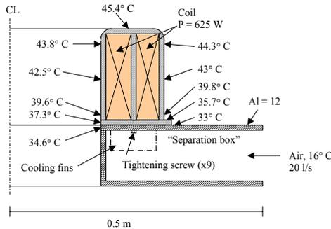
Figure 6: Cross section of the solenoid mounted on the test separation box and the measured steady-state temperatures (after 24 hours) on the surface.
