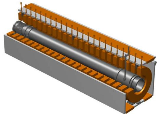
Figure 2: Each straight module on the interaction straight includes: 23 pancake solenoids, four corrector windings, a vacuum chamber with diagnostic unit and bellows.
