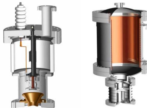
Figure 5: CAD drawings of electron gun (left) and collector (right). The components generating the magnetic field are not shown.
