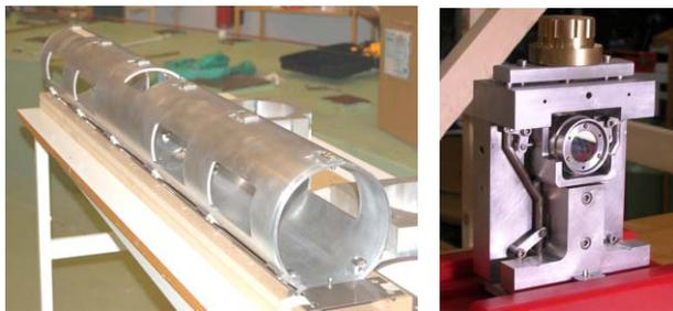
Figure 3: Carriage used for magnetic field measurements (left). Compass based sensor mounted in dedicated holder mechanism (right).
