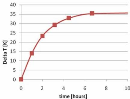
Figure 7: Average coil temperature rise with current 25 A ( $P=625$  W after 8 hours).
