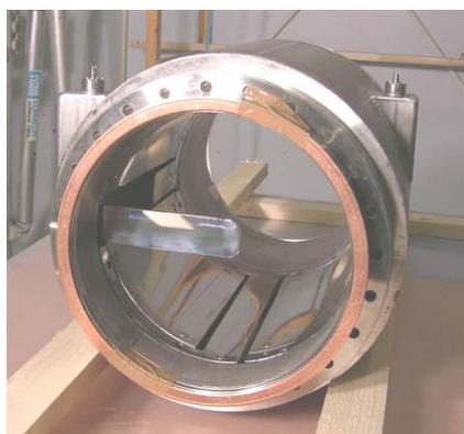
Figure 4: SPUC prototype. (Before the orifice is drilled in the scraper.)
