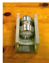
Compass-needle based sensor manufactured by BINP
