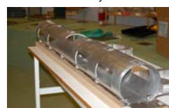
Carriage for magnetic field measurements
