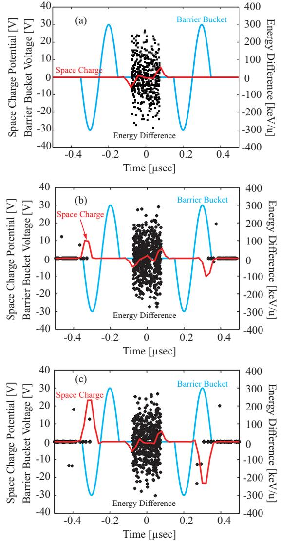
Figure 2: Particle distribution (black dot) in  $\Delta E - \tau$  phase space and barrier bucket voltage (cyan line) and space charge potential (red line), (a) for initial condition (1st injection), (b) for 6th injection, and (c) for 21th injection.
