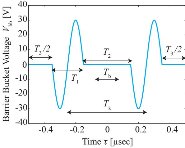
Figure 1: Barrier bucket voltage waveform at each injection time.
