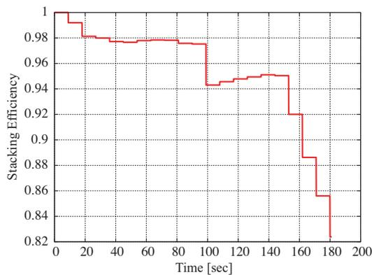
Figure 5: Stacking efficiency (= particle number in the ring / injected particle number).
