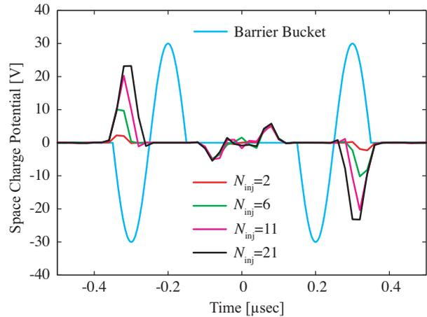
Figure 6: Barrier bucket voltage and space charge potential during the ion storage.
