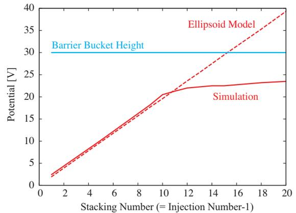
Figure 7: Space charge potential of the analytical estimation and the simulation result.
