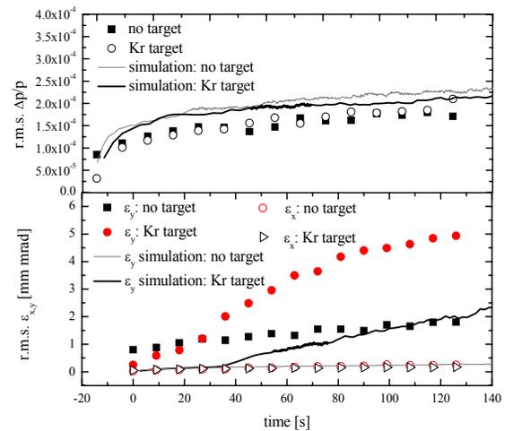
Figure 2: Evolution of  $\Delta p/p$  and  $\epsilon_{x,y}$  for Kr target ( $6 \times 10^{12}$  atoms/cm<sup>2</sup>) compared with BETACOOOL result for an 'effective' density of  $4.36 \times 10^{12}$  atoms/cm<sup>2</sup>.
