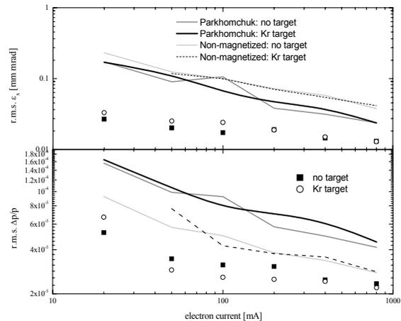
Figure 3: Equilibrium beam parameters compared with BETACOOL simulations using the non-magnetised and Parkhomchuk electron cooling model.
