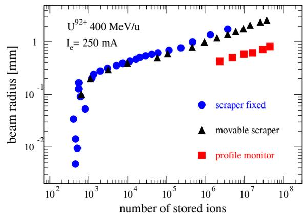
Figure 5: Beam radius measurement of a cooled beam ( $U^{92+}$ , 400 MeV/u) with a residual gas ionization profile monitor ( $1\sigma$ -value), a movable scraper and the method of shifting the ion beam towards the scraper by energy variation of the electron beam.
