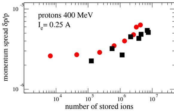
Figure 4: Momentum spread of protons at 400 MeV cooled with an electron current of 0.25 A. The black data points were measured with the standard set-up of the Schottky pick-up at 59.3 MHz, for the red data points the Schottky pick-up was connected to a resonant circuit (29.7 MHz) to increase the signal to noise ratio.
