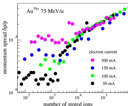
Figure 3: Momentum spread of a bare gold beam at 75 MeV/u cooled with different electron currents. At low intensity the momentum spread depends on the electron current due to the stability of the electron energy.
