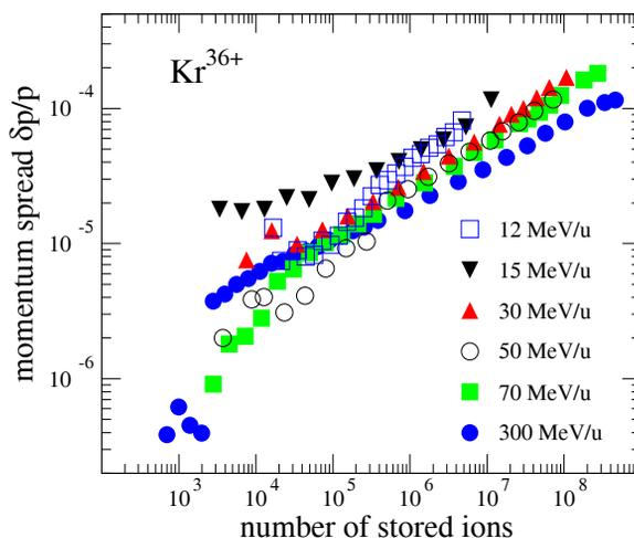
Figure 2: Momentum spread of a beam of bare krypton ions at various energies for an electron density  $n_e = 6 \times 10^6 \text{ cm}^{-3}$ . The stability of the magnetic field of the ring dipole magnets determines the minimum momentum spread at low intensity.
