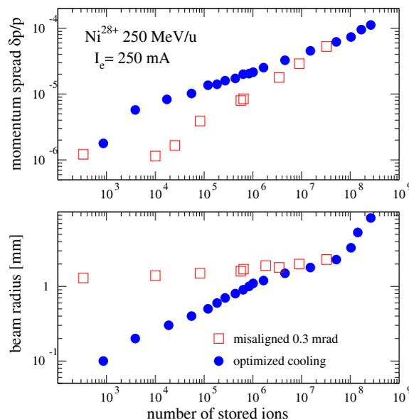
Figure 1: Measurement of the momentum spread and the beam radius of an ion beam ( $^{58}\text{Ni}^{28+}$  250 MeV/u) with perfect alignment of ion and electron beam and with an intentional misalignment of the electron beam by 0.3 mrad. At low intensity the ion beam radius is determined by the misalignment angle, whereas an even smaller momentum spread can be achieved with the misaligned electron beam.
