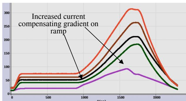
Figure 5: Time evolution of quadrupole currents with corrections to compensate gradients due to ramping.
