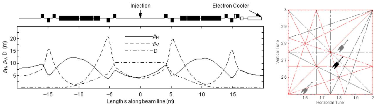
Figure 4: LEIR lattice. The left image shows Twiss parameters for the nominal lattice for one half of the circumference; the right image shows a resonance diagram with the nominal working point (black) and two other envisaged working points. The arrows point from the zero intensity working point to the one with the largest space charge tune shift.
