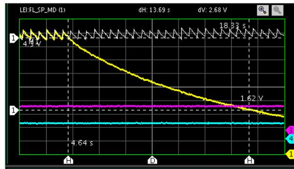
Figure 8: Beam intensity (yellow trace) versus time (2s/div) after accumulation on a very long plateau. The peak intensity is about  $16 \cdot 10^8 \text{ Pb}^{54+}$  ions; and the beam life-time about 14 s.
