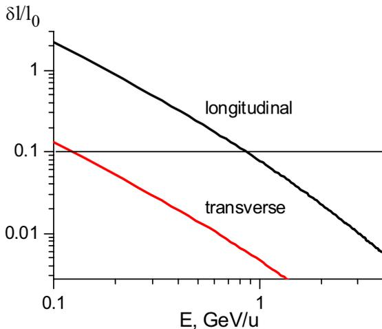
Figure 4: Widening of the kick pulse induced by diverging of two waves. Electron current is  $I_0=0.5$  A, radius of electron beam is  $a=0.5$  cm, frequency bandwidth is  $\Gamma=2$  GHz.
