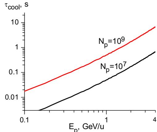
Figure 3: Maximal value of the transverse cooling rate versus energy of the cooled particle.
