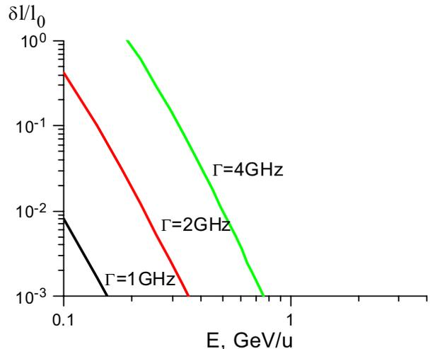
Figure 5: Widening of the kick pulse induced by dispersion of the longitudinal wave. Electron current  $I_0=0.5$  A, radius of electron beam  $a=0.5$  cm, frequency bandwidth  $\Gamma=1, 2$  and  $4$  GHz.
