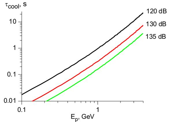
Figure 7: Transverse cooling time versus energy at the different values total amplifier gain. The rest parameters of the estimation are  $N_p=10^9$ ,  $\Gamma=1$  GHz,  $f_0=1$  MHz,  $\rho=50$  Ohm,  $T_{amp}=60$  K,  $L_{cool}=4$  m,  $\beta_{cool}=15$  m,  $Z_{gun}^{-1}=1$  mA/V.
