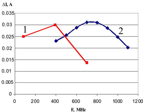
Figure 6: Modulation current versus frequency at 20 V modulation voltage. The curve 1 corresponds to usual BINP electron gun used in EC-35 (CSRm), EC-300 (CSRc), EC-40 (LEIR), curve 2 is variant 1 decreases in scale 2.
