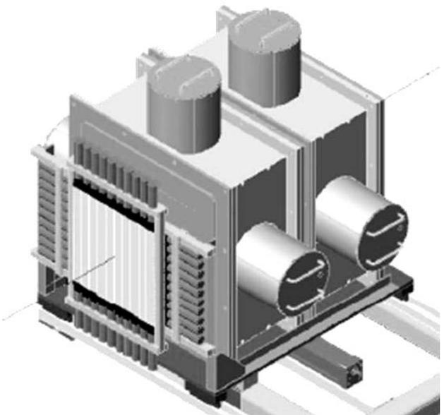
Figure 5: 3-D rendering of the upstream PID module, showing the first TOF station (foreground) and the two Cherenkov counters (background).
