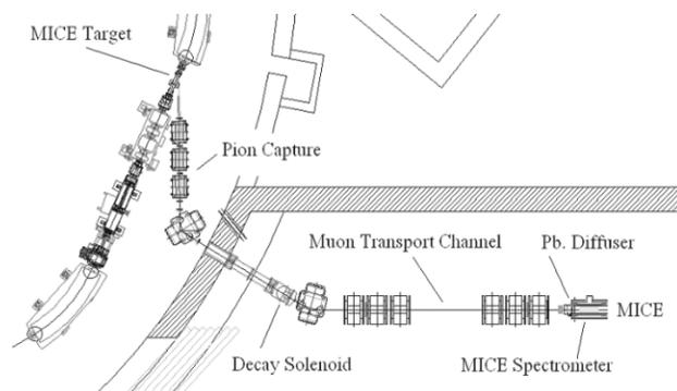
Figure 1: Schematic view of the MICE beam line at ISIS, Rutherford Appleton Laboratory, UK.
