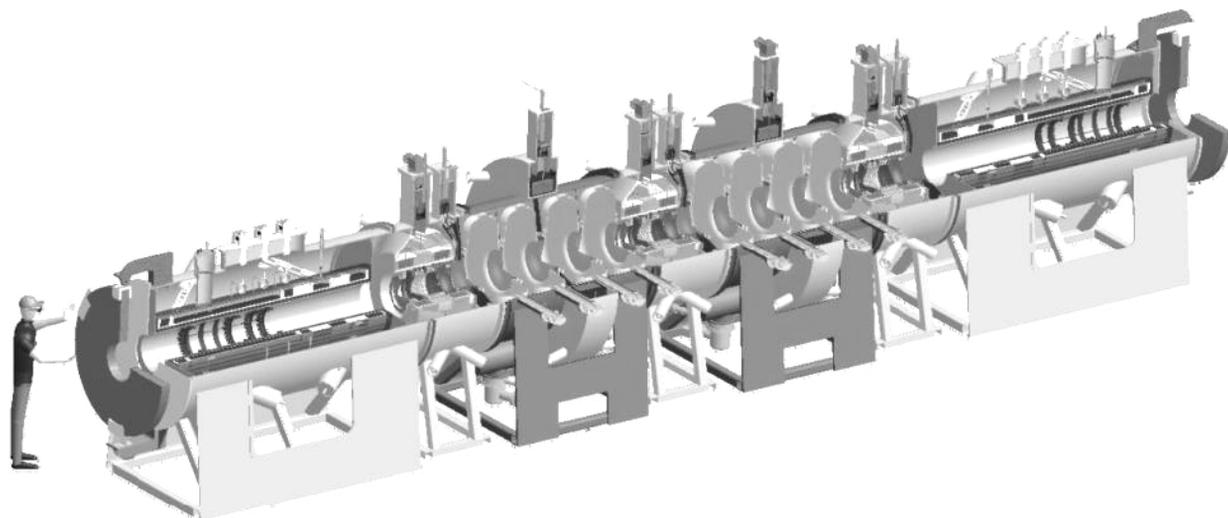
Figure 2: 3-D cutaway rendering of the MICE apparatus, showing, from left to right, the first spectrometer module, the first LH<sub>2</sub> absorber module, the RF module and, at the centre of symmetry, the second absorber module.
