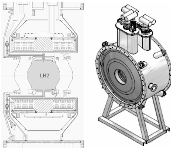
Figure 3: Left: a sketch of the LH<sub>2</sub> absorber. Right: 3D rendering of the Focus Coil Module.
