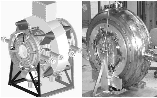
Figure 4: The RF and Coupling Coil Module. Left: three-dimensional rendering of the preliminary design. Right: The prototype 201 MHz RF Cavity.
