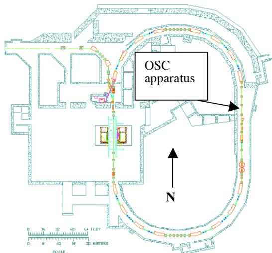
Figure 2: Layout of the South Hall Ring. The OSC experiment will be located in its eastern straight section.
