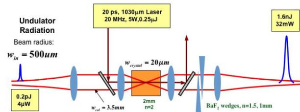
Figure 4: Layout of the optical amplifier.
